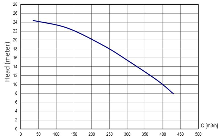
Flow @ 1475rpm (m<sup>3</sup>/hour)
